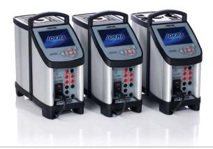
The PTC Series matches lab features like a wide temperature range, high accuracy, stability, and speed. The PTC Series features an active dual zone temperature control which provides excellent temperature homogeneity in the well.
